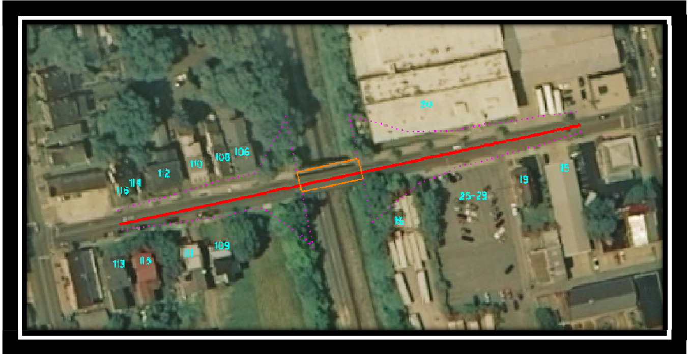
Figure 3 - Preliminary plan view of Alternate 1A. The red line represents the proposed centerline of the new approaches. The orange box represents the proposed bridge, and the purple dotted line shows the approximate disturb limits. The blue numbers depict the addresses of properties along 11 th Street.
